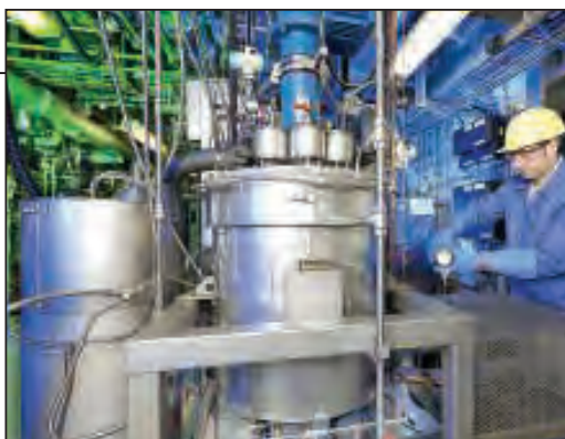
FIGURE 1. This miniplant in Leverkusen, Germany is being used to develop CO 2 -containing polymers for making polyurethane foam used in cars and furniture
